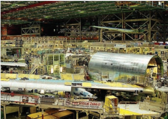
The newer versions – Boeing 777 and the Dreamliner Boeing 787 are presently assembled in four days, and by 2014 they will bring assembling time down to three days with the help of lean tools
